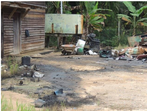
Figure 10: Lubricant and hydraulic oil spillages in one of the plantation visited. Housekeeping of workplace is poor.
