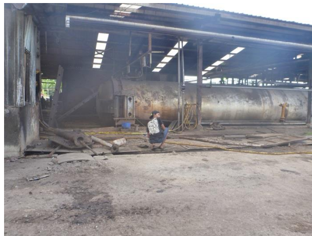
Figure 19: Worker without appropriate PPE and unsafe working condition in a mill.
